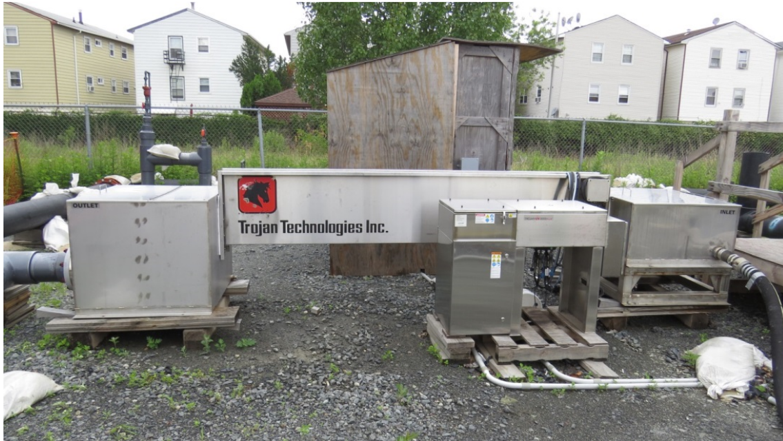
Figure 4.8 Trojan UV3000 unit delivered to site
